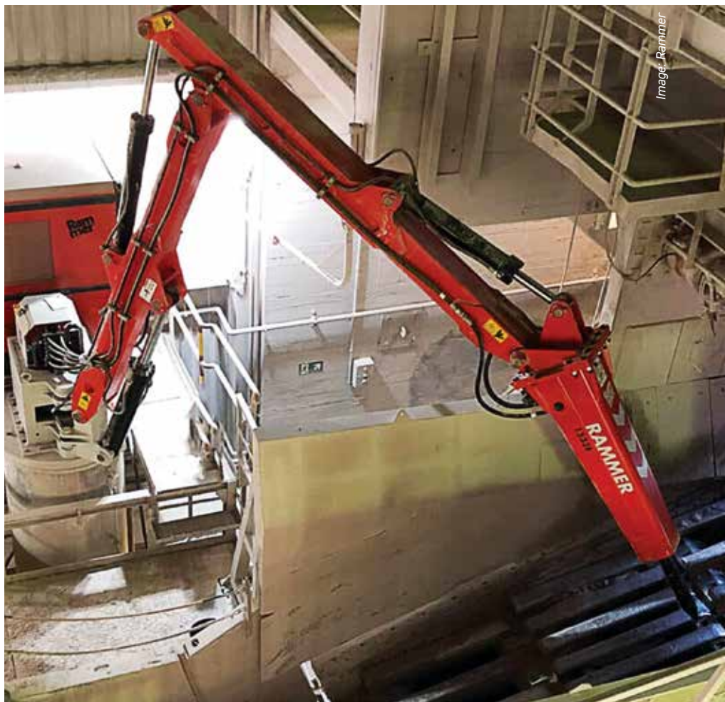
The Rammer Boom System is designed to deal with oversized material.
