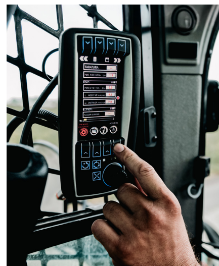
Above: The interface displays real-time data on the asphalt regeneration process, displaying crucial information and enhancing operator connectivity with the equipment.
