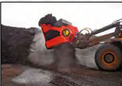
Aerating sludge compost
