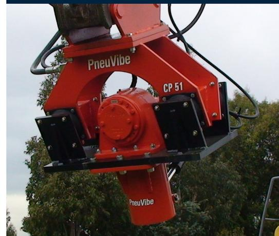
With clamping devices you can effectively combine sheet and perform pile driving in certain soil conditions.
